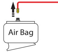
Insert a street tee fitting into the top of the air bag that matches the thread size of the vehicle suspension. Reinstall the suspension air line and fitting into the street tee. For more information on the parts needed for air line installation, see Appendix A.
