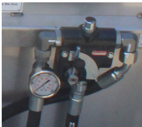
Figure 117 Double Spool Valve for Dual Door Control, Flipper Valve for Pneumatic Door Latch Also Shown
