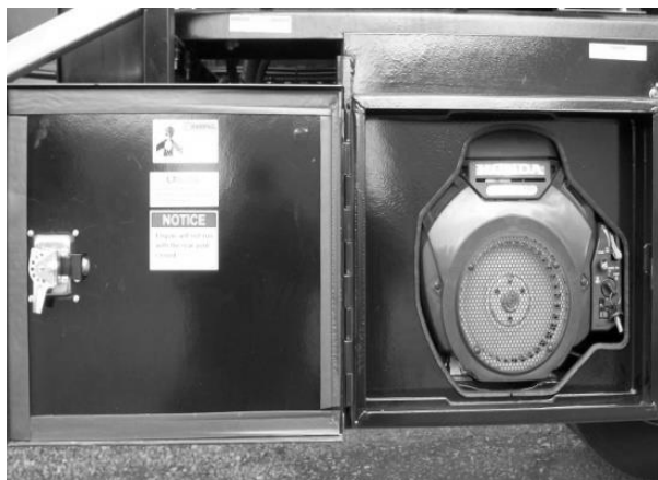
Figure 110 20 HP Gas Engine (Shown in Optional Enclosure)
