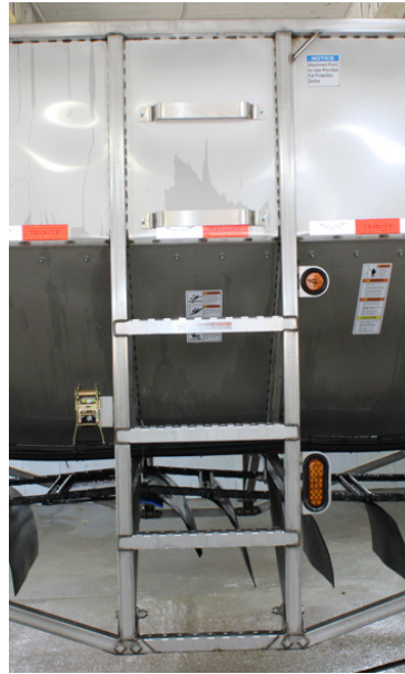
Figure 160 Road Side Ladder Showing Weld on Rungs
