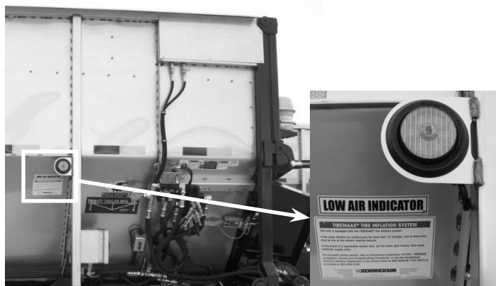
Figure 81 Tire Inflation System Indicator Lamp
