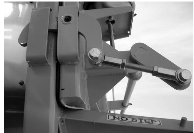
Figure 107 Top Hinge Pneumatic Latch Disengaged
