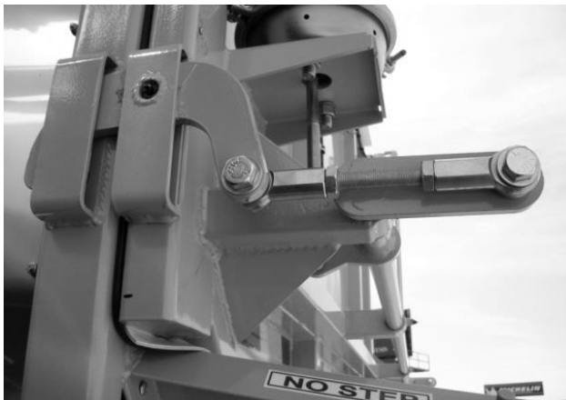
Figure 106 Top Hinge Pneumatic Latch Engaged
