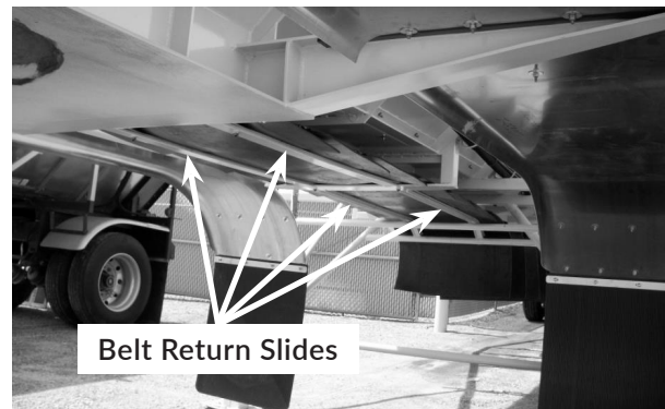
Figure 4 Belt Return Slides Part #F-00149
