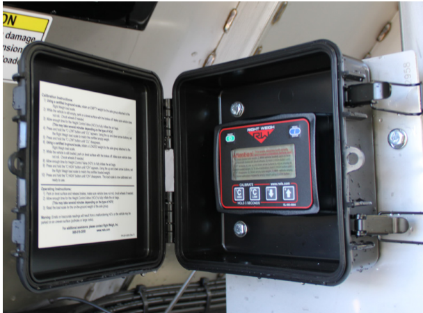
Figure 69 Right-Weigh™ Part #003590 Single, #003649 Dual Registration Box: Part #00087
