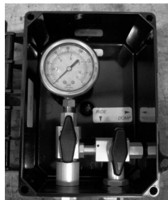
Figure 63 Pneumatic Dump Valve – Part #003653
