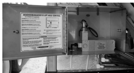
Figure 71 AKAD2010 Lift Control – Part #004231
