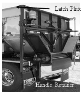
Figure 145 Shur-Lok® Roadside Hardware. Latch Plate: Part #004742
