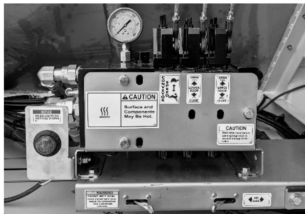
Figure 119 LX6 Manifold with Wet Seal and Air Lock Flipper Valves
