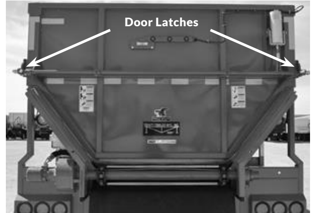
Figure 105 Top Hinge Pneumatic Latches
