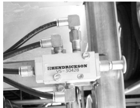
Figure 62 Manual Dump Valve – Part #004228
