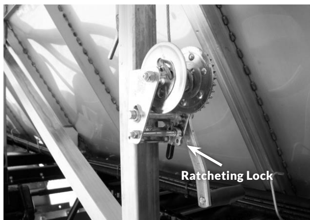
Figure 133 Fold-Down Sideboard Operator Winch Part #001602
