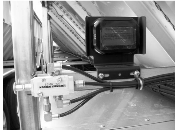
Figure 70 Air-Weigh® QuickLoad™ Part #F-00324 Manual Dump Valve part #004228 pictured lower left
