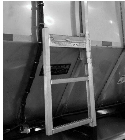
Figure 162 Maintenance Ladder “Stowed” Position
