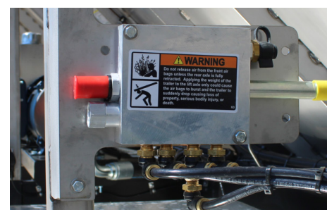
Figure 72A LSAS Lift Control – Part #003848
