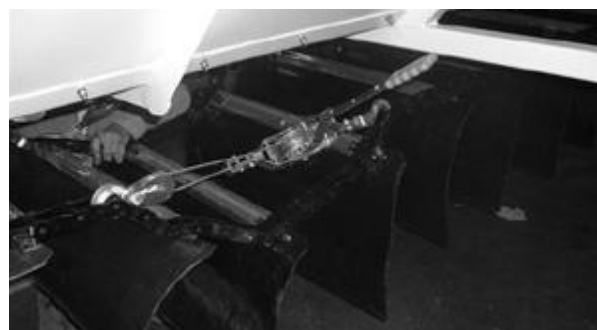
Figure 8 Using Come-Along to Pull Up Chain Slack
