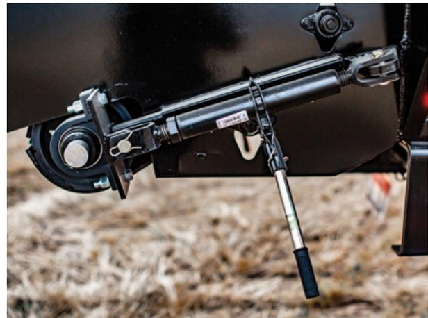
Figure 11 Continuous Belt Adjuster Ratchets
