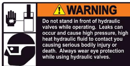
[Figure 26](#) Hydraulic Pressure Leak Warning Label
