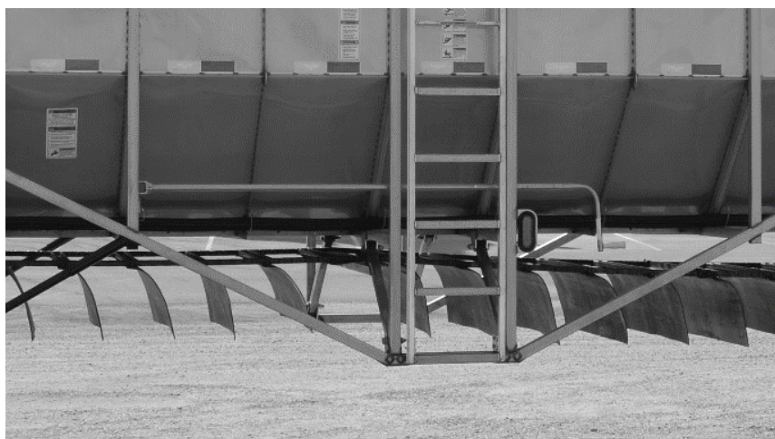
Figure 143- Rollover Tarp Handle Stored.
