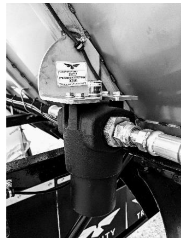
Figure 3- High Pressure Filter Location
