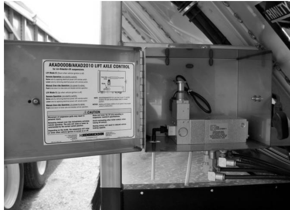
Figure 71- AKAD2010 Lift Control - Part #004230
