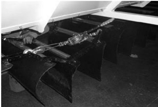
Figure 8 - Using Come-Along To Pull Up Chain Slack
