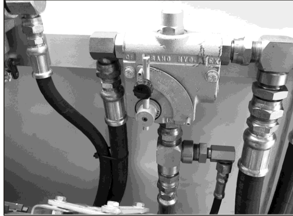
Figure 114- Flow Control Used to Control Belt in PTO Systems. - Part #004402
