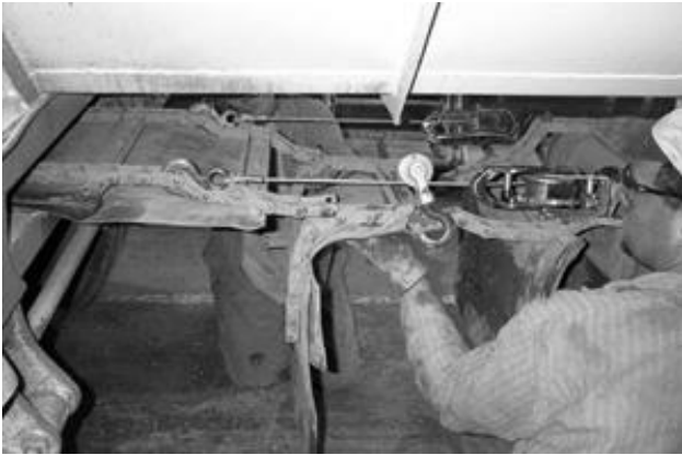
Figure 9- - Determine How Much Chain to Remove
