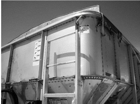
Figure 158- Front Ladder Showing Upper User Fall Protection Device.
