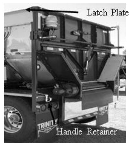
Figure 145- Shur-Lok® Roadside Hardware
