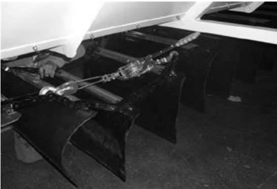
Figure 6 - Using Come-Along To Pull Up Chain Slack
