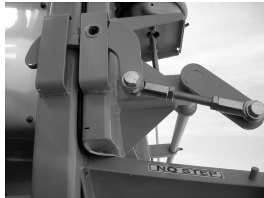
Figure 104- Top Hinge Pneumatic Latch Disengaged.
