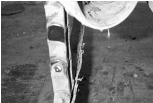
Figure 8- Chain Pin with Head Ground Off
