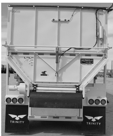
Figure 91 - Hydraulic Lift Top-Hinge with Hydraulic Flip-Up Door
