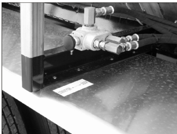
Figure 108 - Push-Pull Valve Used to Select Door or Belt Control
