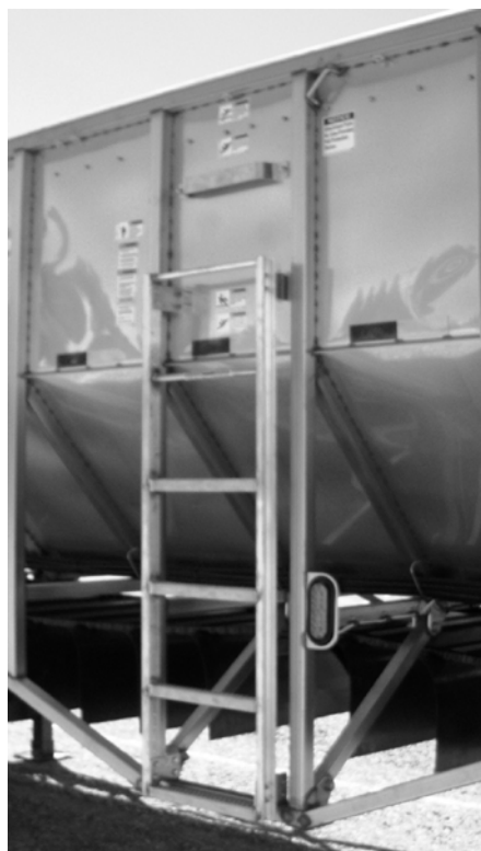
Figure 155 - Roadside Ladder Showing Offset
