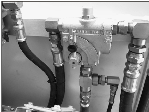
Figure 107 - Flow Control Used to Control Belt in PTO Systems
