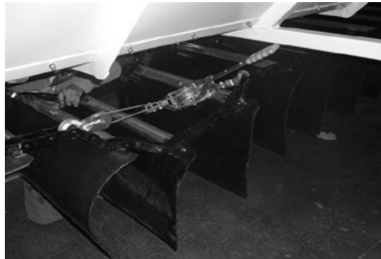
Figure 6 - Using Come-Along To Pull Up Chain Slack
