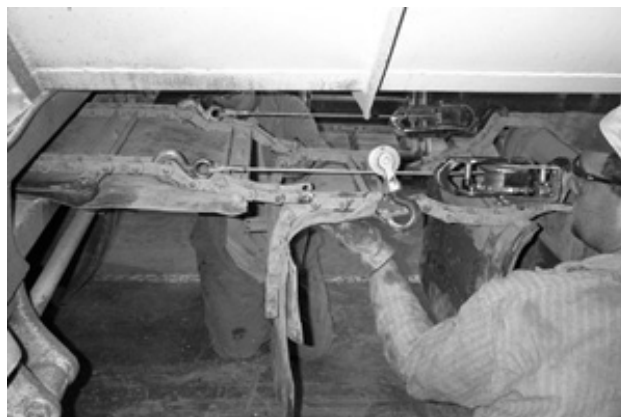
Figure 6 - Using Come-Along To Pull Up Chain Slack
