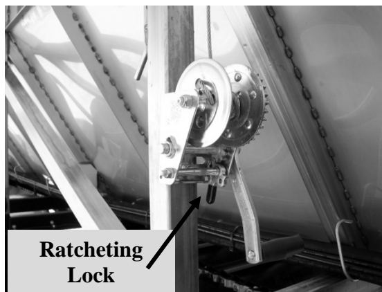
Figure 128 - Fold-Down Sideboard Door Operator Winch
