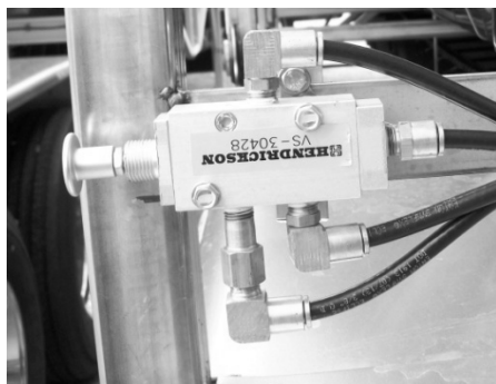
Figure 54 - Dump valve used with electronic scale
