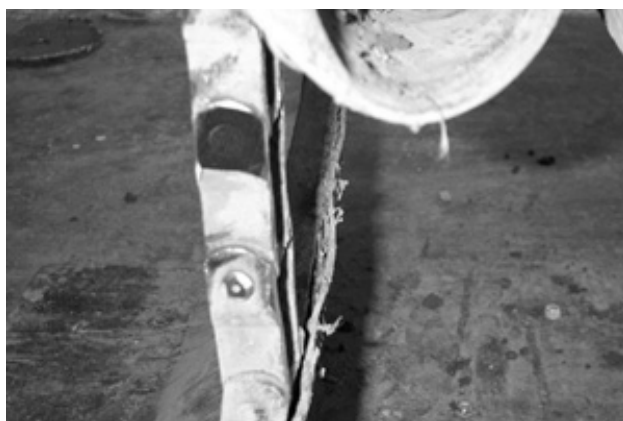
Figure 8 - Chain Pin with Head Ground Off
