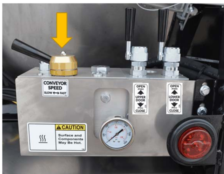
Figure 111 - Manifold - Arrow Indicates the Conveyor Flow Control
