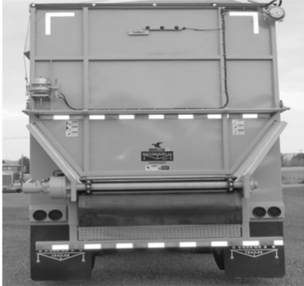
Figure 89 - Pneumatic Lift Top-Hinge with No Lower Door
