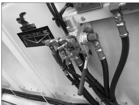
Figure 109 - Single Door Valve for Door Control
