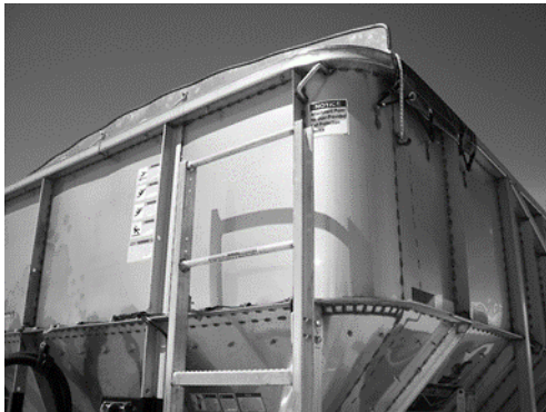
Figure 153 - Front Ladder Showing Upper User Fall Protection Device
