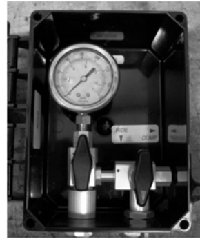
Figure 55 - Dump valve used with air gauge
