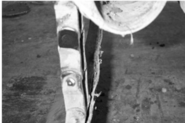
Figure 8 - Chain Pin with Head Ground Off
