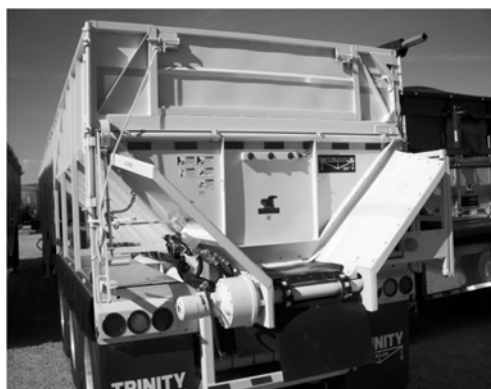
Figure 84 - Full Swing "Spud" With Manual Flip-Up Door
