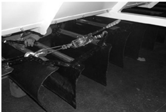
Figure 6 - Using Come-Along To Pull Up Chain Slack
