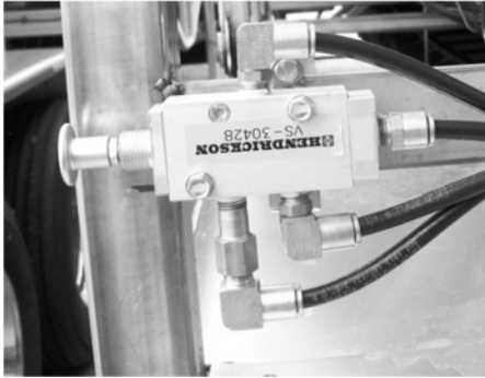
Figure 54 - Dump valve used with electronic scale
