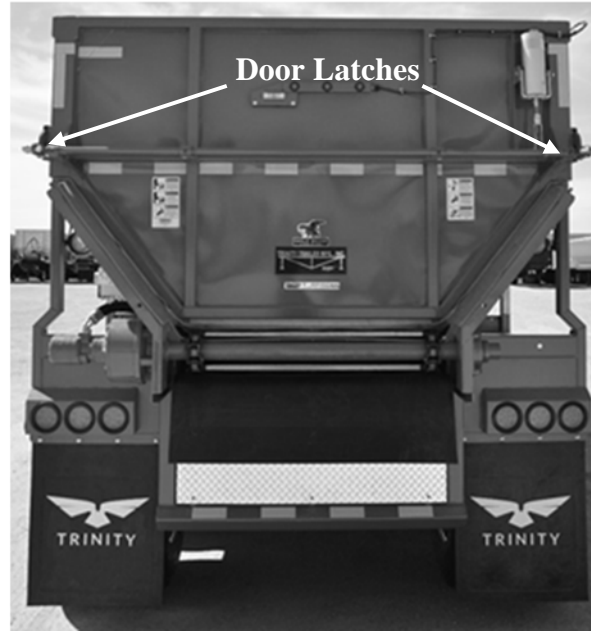
Figure 98 - Top Hinge Pneumatic Latches
