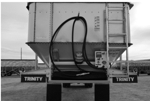
Figure 133 - Pneumatically-Actuated Front Wet Seal
