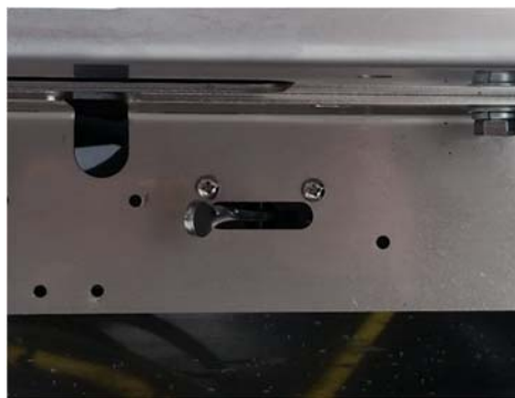
Figure 134 -Control Valve for Pneumatically- Actuated Front Wet Seal located under the manifold.
