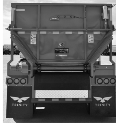
Figure 90 - Hydraulic Lift Top-Hinge with No Lower Door
