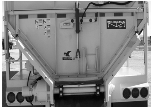
Figure 78 - Hydraulic Flip-Up Lower Door
