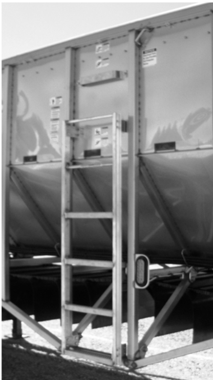
Figure 155 - Roadside Ladder Showing Offset
