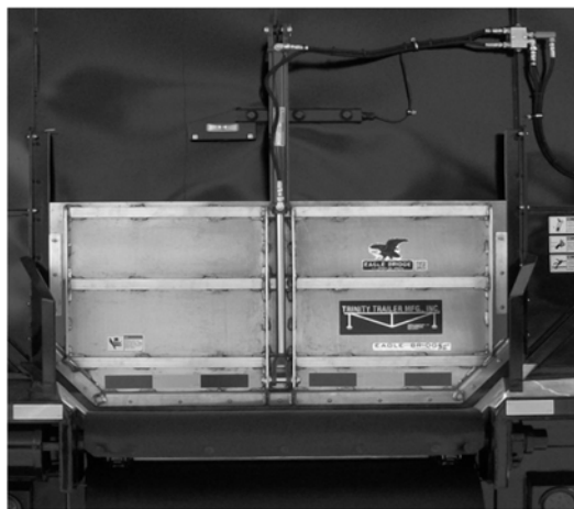
Figure 80 - Hydraulic Slide-Up Lower Door
