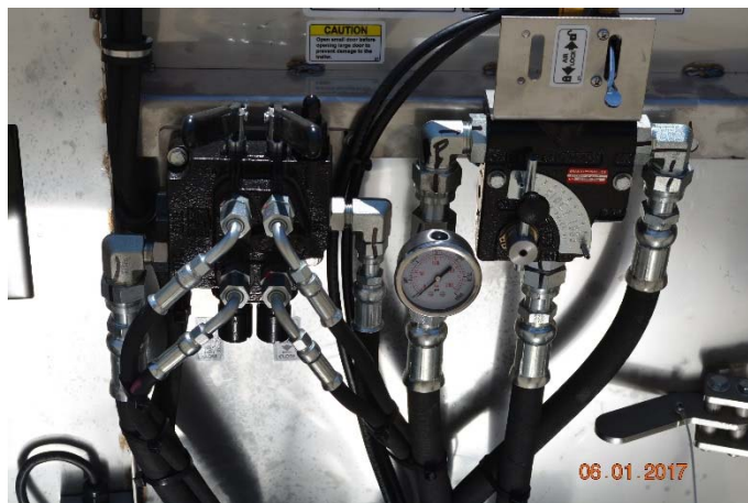
Figure 110 - Double Spool Valve for Dual Door Control, Flipper valve for Pneumatic Door Latch also shown.
