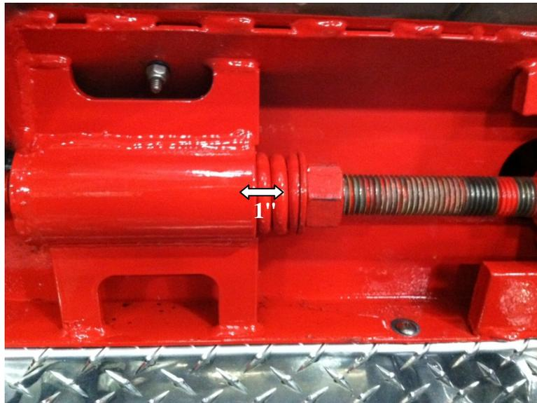
**Figure 4 - Chain Adjustment**
