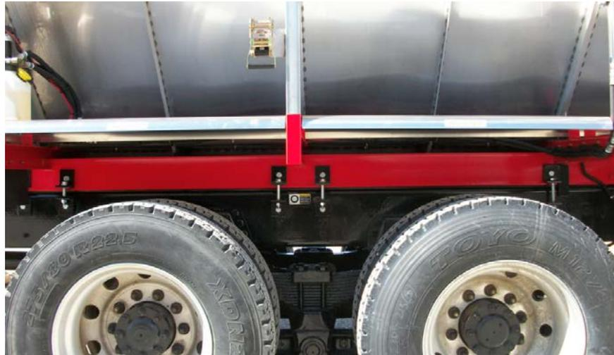
**Figure 3-Center Mounting Brackets (typical)**
