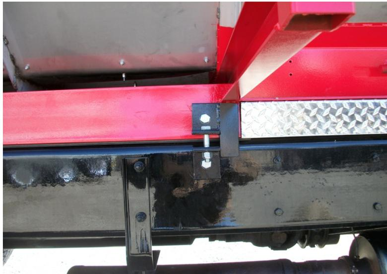
**Figure 1-Front Mounting Brackets (typical)**
