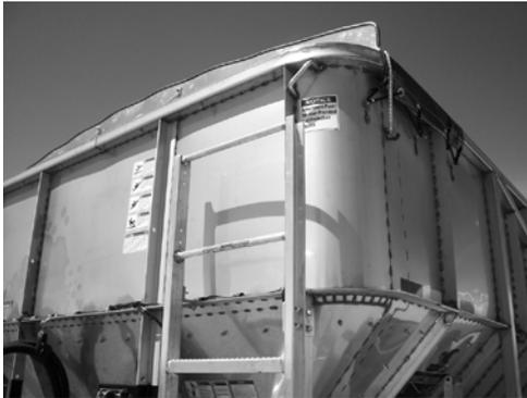
**Figure 147 - Front Ladder Showing Upper User Fall Protection Device**
