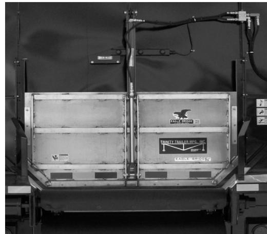
**Figure 79** - Hydraulic Slide-Up
