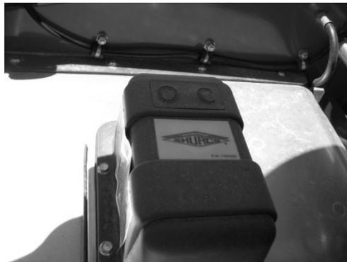
Figure 136 - Electric Tarp Rocker Switch
