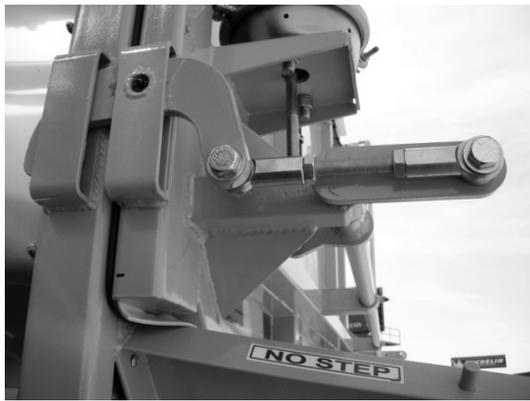
**Figure 98 - Top Hinge Pneumatic Latch Engaged**
