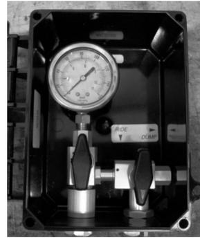
**Figure 53** - Dump valve used with air gauge
