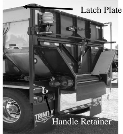
Figure 133 - Shur-Lok® Tarp Rolled Up
