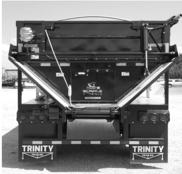
**Figure 92 - Hydraulic Lift Top-Hinge "Spud" With Hydraulic Flip-Up Door**
