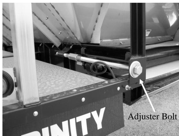
Figure 4 - Chain Adjustment Assembly
