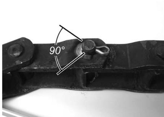
Figure 9 - Properly Welded Pin
