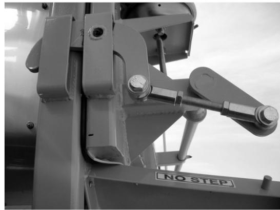
**Figure 99 - Top Hinge Pneumatic Latch Disengaged**
