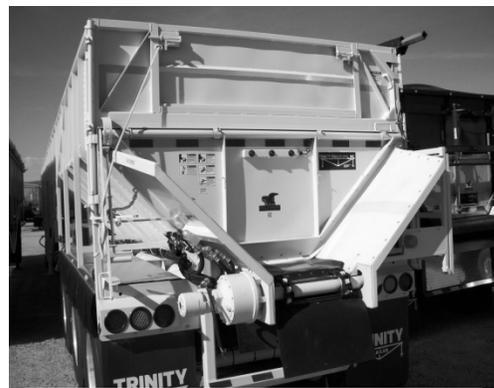
**Figure 83 - Full Swing "Spud" With Manual Flip-Up Door**
