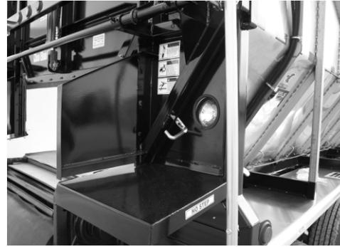
**Figure 101-** Slide-Up Door Clamp Latch Disengaged
