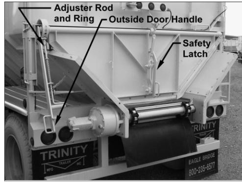
**Figure 81 - Manual Flip-Up Door Components**
