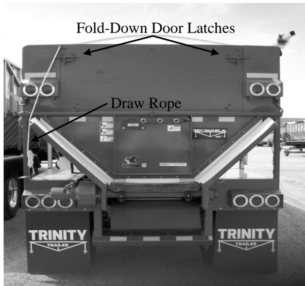
**Figure 93 - "Spud" Door Components**
