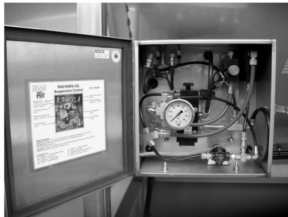
**Figure 65 - RA016SRA-32L Suspension Control**
