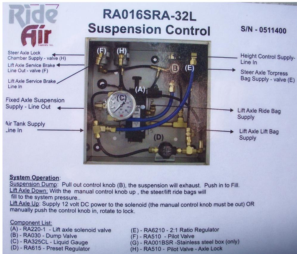
**Figure 66 - Suspension Control Components and Locations**
