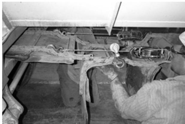
Figure 7 - Determine How Much Chain to Remove
