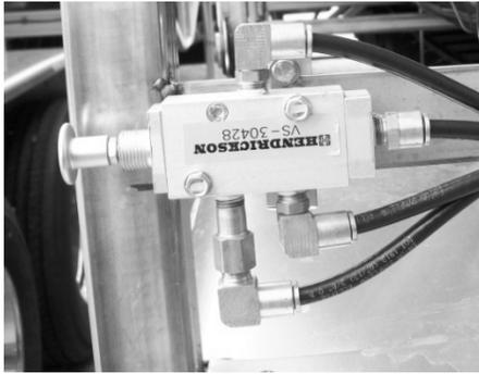
**Figure 52** - Dump valve used with electronic scale
