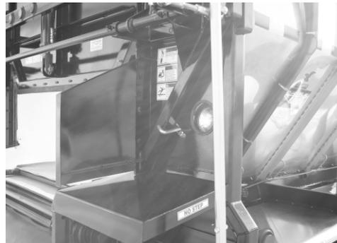
**Figure 100 - Slide-Up Door Clamp Latch Secured**
