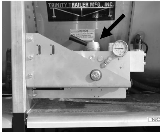
Figure 105 - Manifold - Arrow Indicates the Conveyor Flow Control
