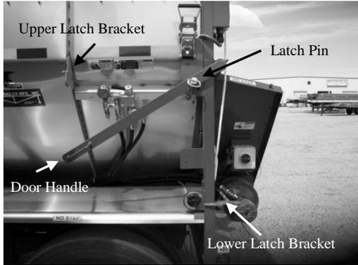
**Figure 80 - Manual "Spud" Door Components**
