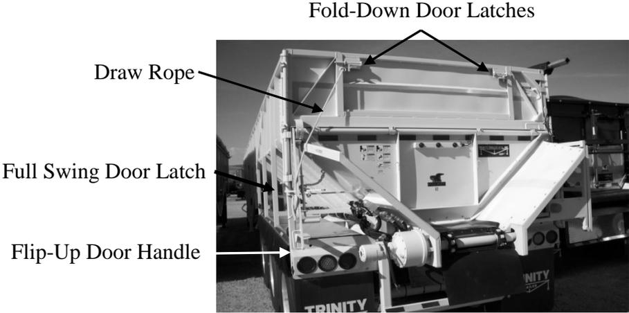
**Figure 94 - Full-Swing “Spud” Door Components**
