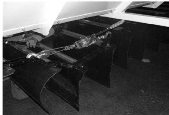
Figure 6 - Using Come-Along To Pull Up Chain Slack
