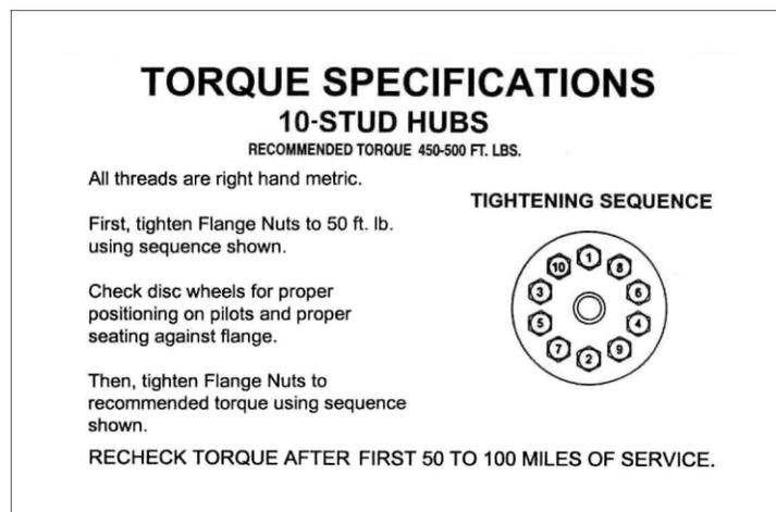
Figure 39 - Pilot Mount Wheel Torque Specifications
