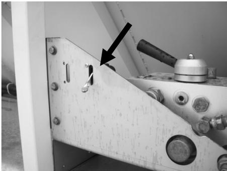
Figure 108 - Flipper Valve for Pneumatic Door Latch
