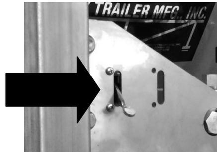
**Figure 128** - Control Valve for Pneumatically-Actuated Front Wet Seal
