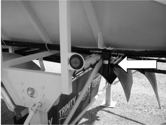
**Figure 40** - Pressure Filter Location
