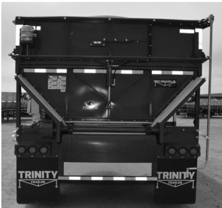
**Figure 90 - Hydraulic Lift Top-Hinge
