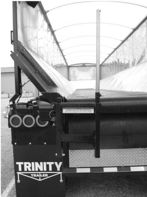
**Figure 155 - Telescoping Handle Extended**
