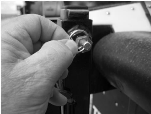
**Figure 153 - Telescoping Handle Release Pin**
