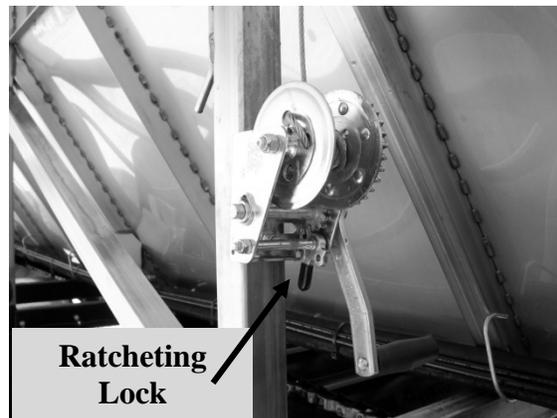
**Figure 122** - Fold-Down Sideboard Door Operator Winch
