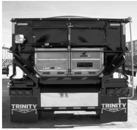
**Figure 91 - Hydraulic Lift Top-Hinge
