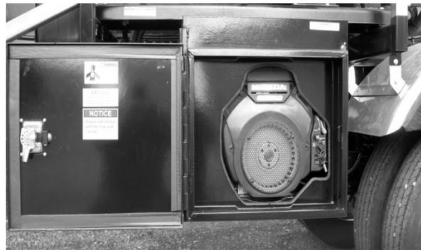
**Figure 102 -** 20 HP Gas Engine
