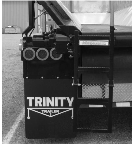
**Figure 156 - Maintenance Ladder In Use Position**
