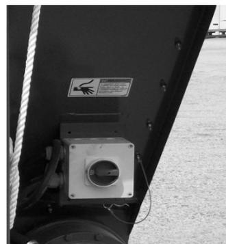
**Figure 104 -** Electric Motor Power Switch
