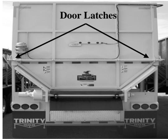
**Figure 97 - Top Hinge Pneumatic Latches**
