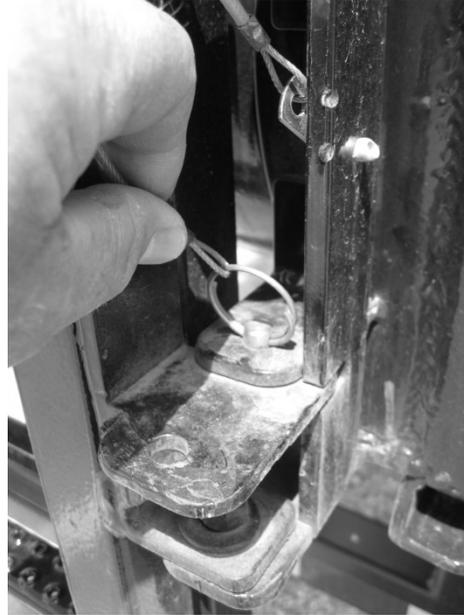
**Figure 152 - Position Locking Pin**
