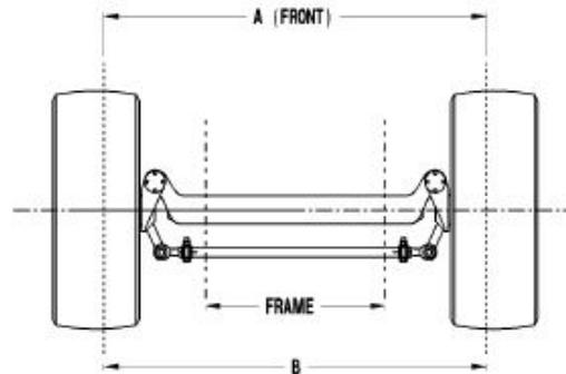
1. Tires must be of the same size, pressure, and tread pattern. Hubs, drums and brakes must be identical. All suspension bushings and parts must be in good mechanical order and correctly adjusted.
